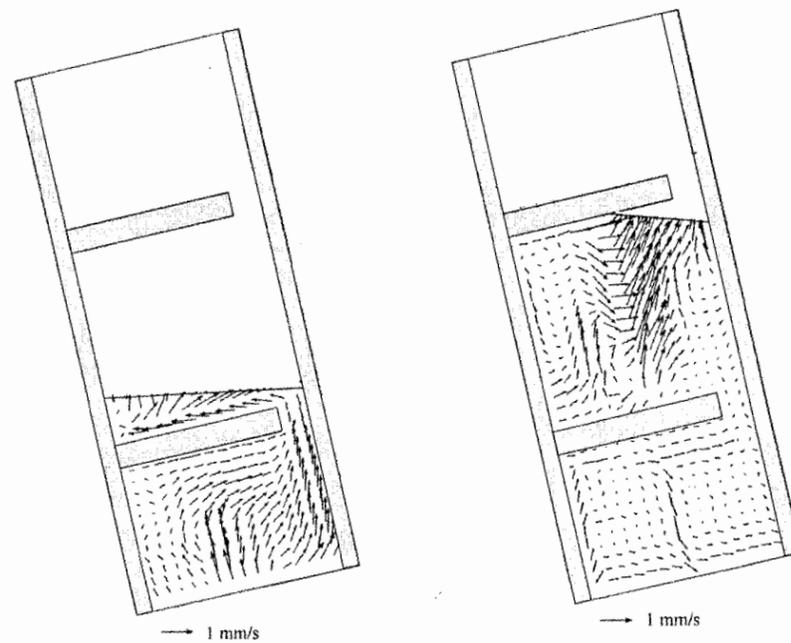
Figure 2: PIV evaluated velocity fields for cavity inclined at 13.5°; fluid passing the first (left) and the second obstacle (right).
