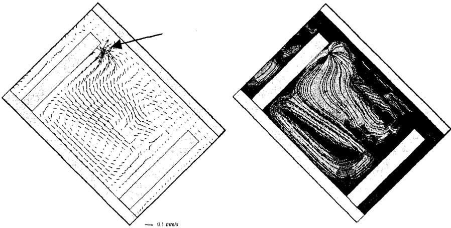
Figure 5: PIV evaluated velocity field (left) and streamlines integrated for this field with colour coding of velocity value (right) ; middle section of the cavity observed 180s after closing the inlet; shrinkage of liquid at the “hot spot”; inclination of the cavity  $45^\circ$ .
