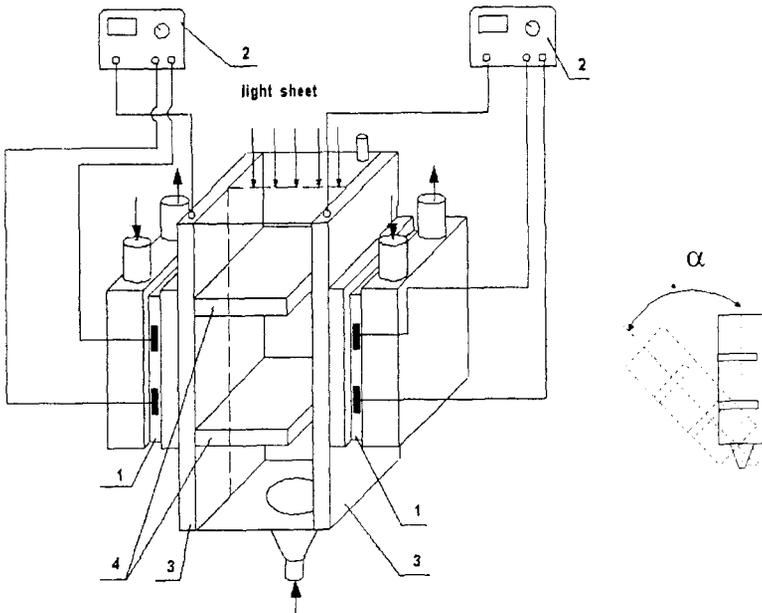
Figure 1: Schematic of the experimental system. 1 – Peltier elements, 2- controllers, 3- isothermal walls of the cavity, 4 – inner obstacles.
