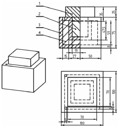
Figure 1: Scheme of cubic container (SIG) made of Plexiglas with cooling liquid layer:
