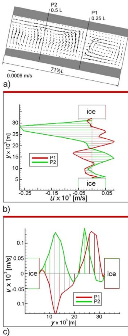
Figure 5: Measurements in freezing water – results registered after 974s: a) velocity field; b), c) velocity profiles (Table 2, #40)
