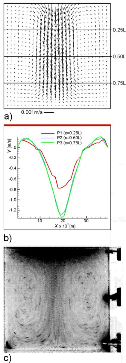
Figure 4: Velocity field (a), velocity profiles (b) and particle tracks (c) observed during stationary natural convection (Table 2, #18)
