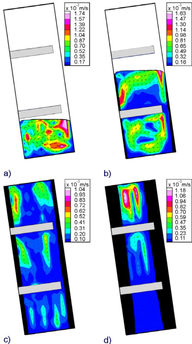
Figure 6: Evolution of velocity contours and ice volume growth in freezing water after: a) 17s, b) 45s, c) 267s, d) 1163s (Table 2, #47)
