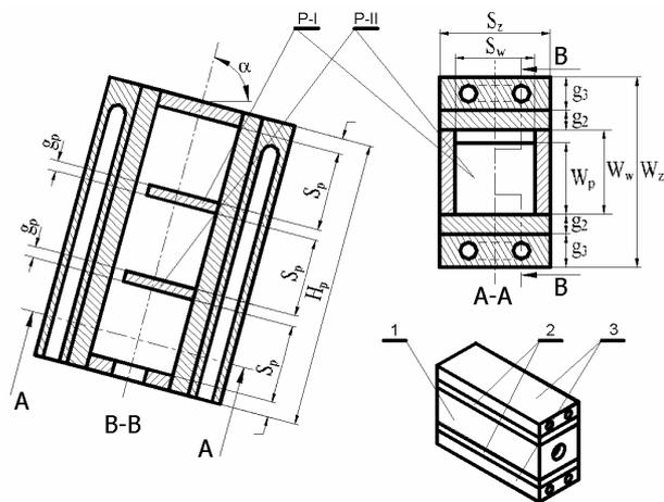
Figure 2: Scheme of rectangular channel (PZP):
