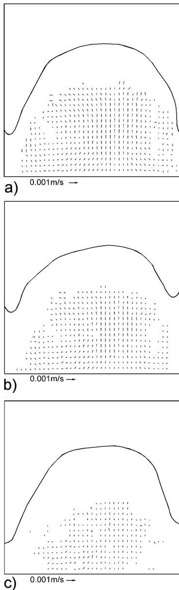
Figure 3: Velocity fields and phase transformation front evolution (Table 2, #6)
