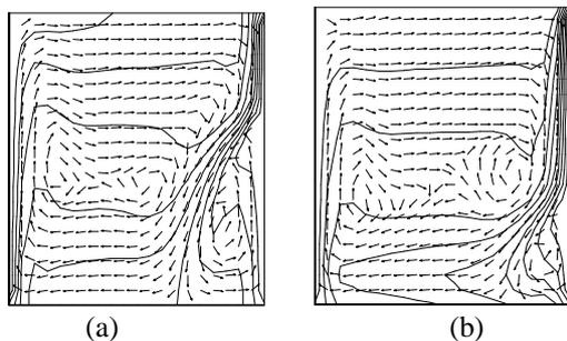
Fig. 5. Natural convection of water, numerical results for  $T_h=10^\circ\text{C}$ ,  $T_c=0^\circ\text{C}$ ,  $Ra=1.5 \cdot 10^6$ ,  $Pr=13.3$ . Velocity and temperature fields in the centre plane ( $z=0.5$ ). Effect of *TBC*; (a) - adiabatic, 1-D *TBC*, (b) - non-adiabatic, 3D-*TBC* with  $d/L=0.167$ .
