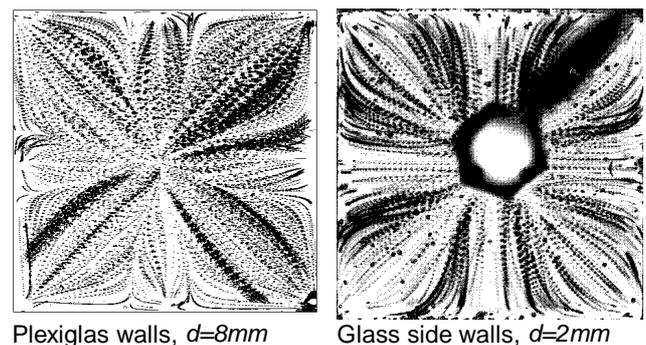
Fig. 7 Natural convection of water in lid cooled cavity:  $T_h=21^\circ\text{C}$ ,  $T_c=15.5^\circ\text{C}$ ,  $Ra=2.7 \cdot 10^6$ . Particle tracks observed underneath the lid for plexiglas (left) and glass (right) passive walls of the cavity.
