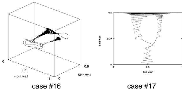
Fig. 3. Calculated streamlines for non-adiabatic *TBC* (case #16 and #17 in Table 1b). Right figure: 1-D *TBCs* used, unable to predict observed splitting of the spirals. Additional saddle points close to the centre plane ( $y=0.35$ ) divide the spirals into two, running in opposite directions; this was not observed in the experiments. Left figure: 3D-*TBCs* correctly predict splitting of the spirals and their direction (to the centre).
