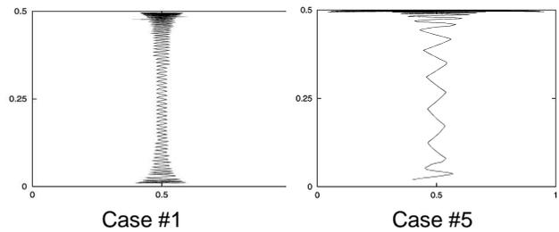
Fig. 2. Calculated streamlines in the horizontal centre plane ( $y=0.5$ ) for adiabatic *TBC*. The tracks run from the front wall (bottom of the figures) to the cavity centre. Effect of the side wall thickness on a pitch of the tracks (case #1 and #5 in Table 1a).
