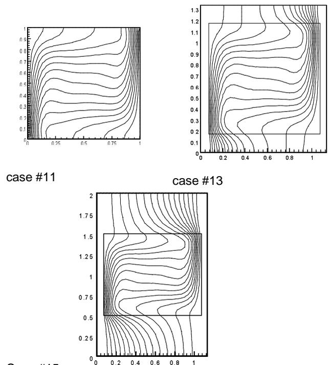
Fig 4. Isotherms calculated for the centre plane ( $z=0.5$ ); case #11, #13 and #15 in Table 1b. Effect of the side wall thickness for adiabatic *TBC*:  $d/L=0$  (left),  $d/L=0.167$  (right),  $d/L=0.5$  (bottom).
