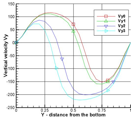
Fig. 6 Natural convection of water (parameters like Fig. 5). Vertical velocity profiles calculated close to the cold wall (vertical line at  $x=0.93$ ,  $z=0.5$ ) for 1D-*TBC*. Effect of the heat flux through the side walls:  $Vy_0$  - adiabatic,  $Vy_1$  -  $h=2\text{W/Km}^2$ ,  $Vy_2$  -  $h=20\text{W/Km}^2$ ,  $Vy_3$  -  $h=40\text{W/Km}^2$ . Zero crossing of the profiles indicates position of the saddle point of the colliding hot-cold circulations.
