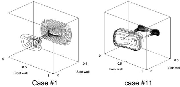
Fig. 1. Calculated 3-D streamlines (front half of the cavity displayed only) for adiabatic *TBC* (case #1 and #11 in Table 1). One or two straight spirals run towards centre (case #1) or towards front wall (case #11).
