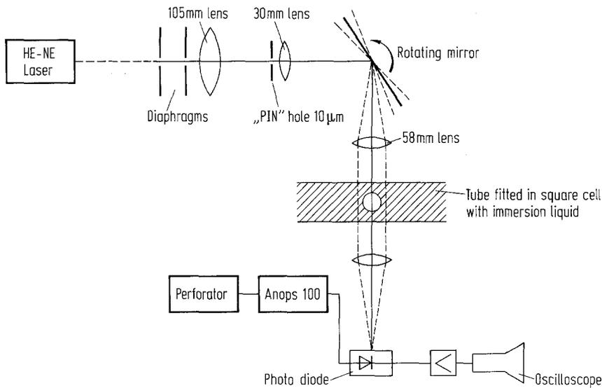
Fig. 3. The optical system for concentration measurements
