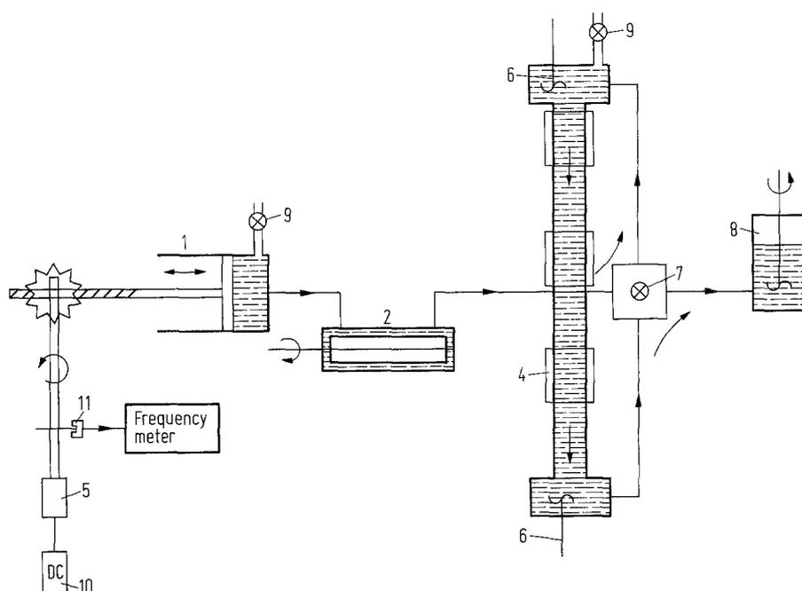
**Fig. 1.** The flow system: 1 pump; 2 Couette mixer; 3 flow tube; 4 cell with immersion liquid; 5 motor; 6 stirrer; 7 valves; 8 tank with breaker; 9 air valves; 10 reg. d.c. power supply; 11 revolution meter
