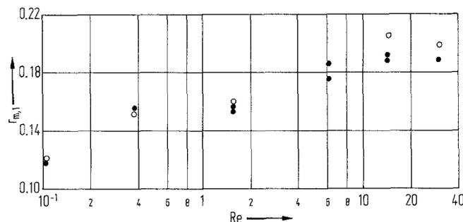
Fig. 7. The relative distance from the wall of the side maximum as a function of the Reynolds number:  $\lambda = 0.15$ ,  $\bar{a} = 0.01$ ,  $c_s = 0.05$ . Closed circles:  $\bar{x} = 10$ ; open circles:  $\bar{x} = 80$
