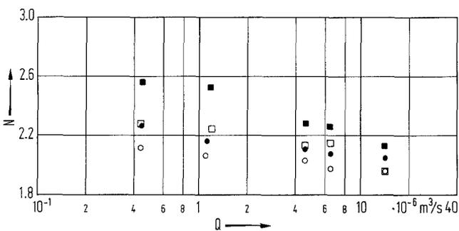
**Fig. 9.** Velocity profile blunting parameter vs. flow rate:
