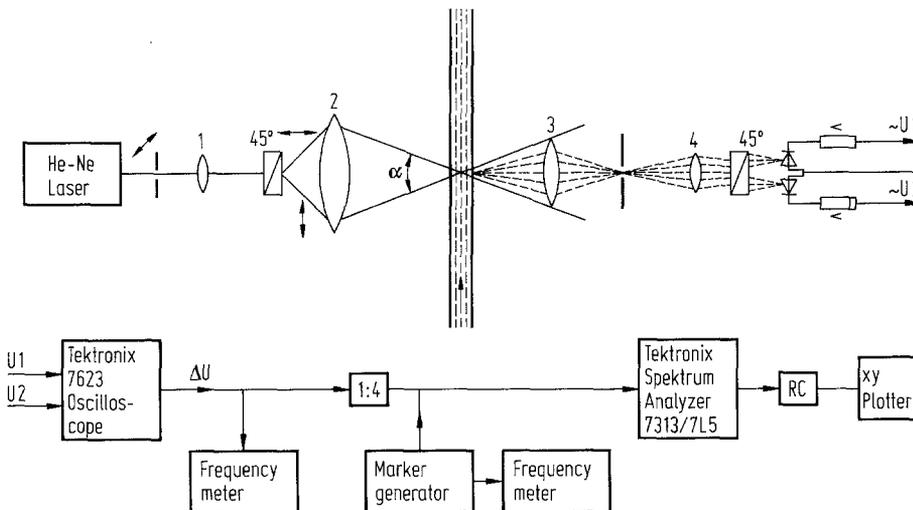
Fig. 4. The Laser-Doppler system
