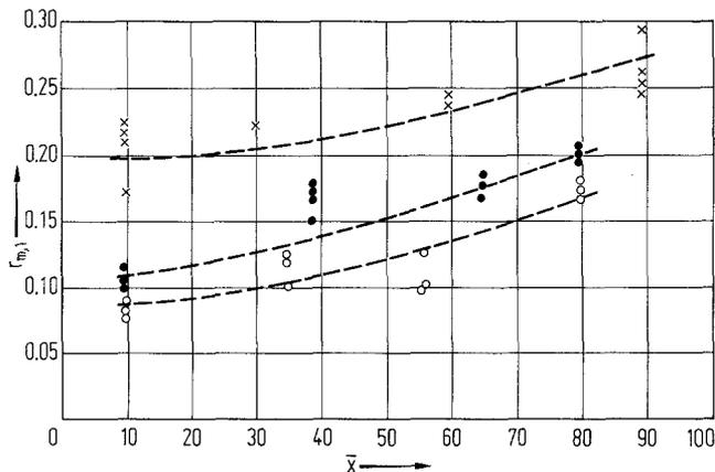
Fig. 6. The relative distance from the wall of the side maximum as a function of the distance from the tube inlet:
