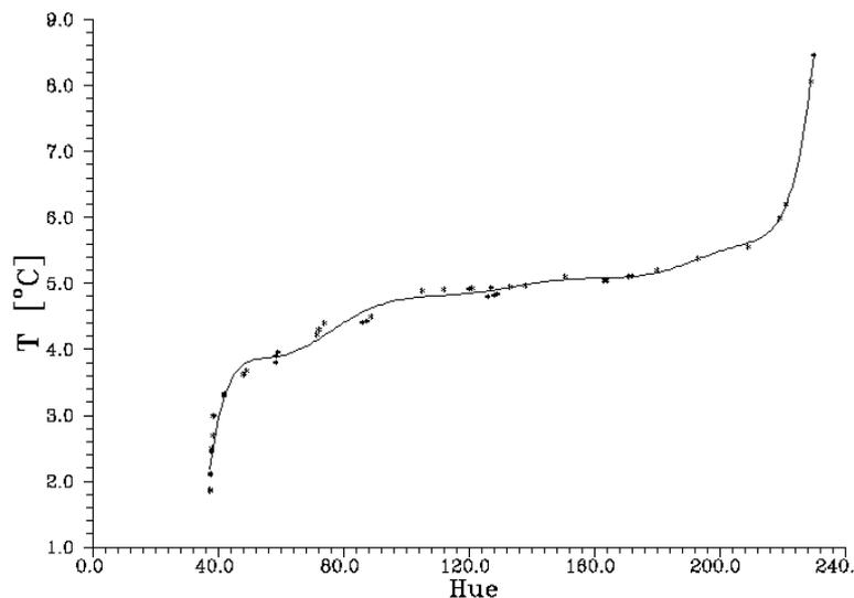
**Figure 2.** Temperature vs. Hue for TLCs sample used to study natural convection of water with freezing. Calibration curve obtained by 8<sup>th</sup> order polynomial fitted to the experimental points
