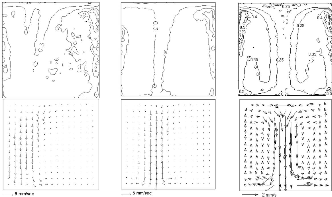
**Figure 11.** Typical instabilities observed during the onset of convection: temperature (upper row) and velocity (bottom row) fields measured by DPIV &  $T$  for the centre plane of the cube shaped cavity made of plexiglas;  $T_h=21^{\circ}\text{C}$ ,  $T_c=15^{\circ}\text{C}$ ,  $Ra=2.7 \cdot 10^6$ ,  $Pr=8$
