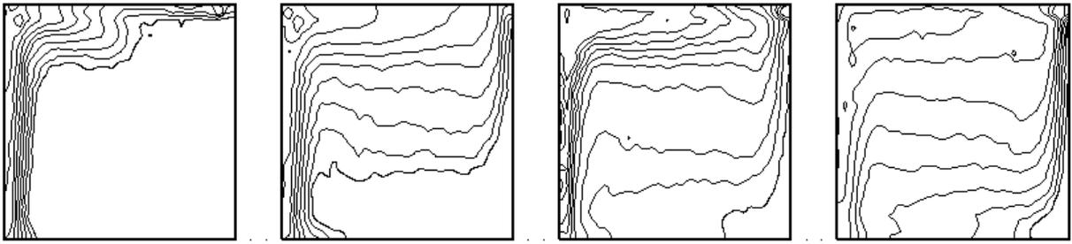
**Figure 8.** Transient development of isotherms measured at the centre-plane of differentially heated cavity: time  $t=2\text{min}$ ,  $10\text{min}$ ,  $20\text{min}$  and  $60\text{min}$  after the temperature  $T_h$  is applied; initial fluid temperature  $T_o = T_c$ ;  $Ra=1.8 \cdot 10^5$ ,  $Pr=980$
