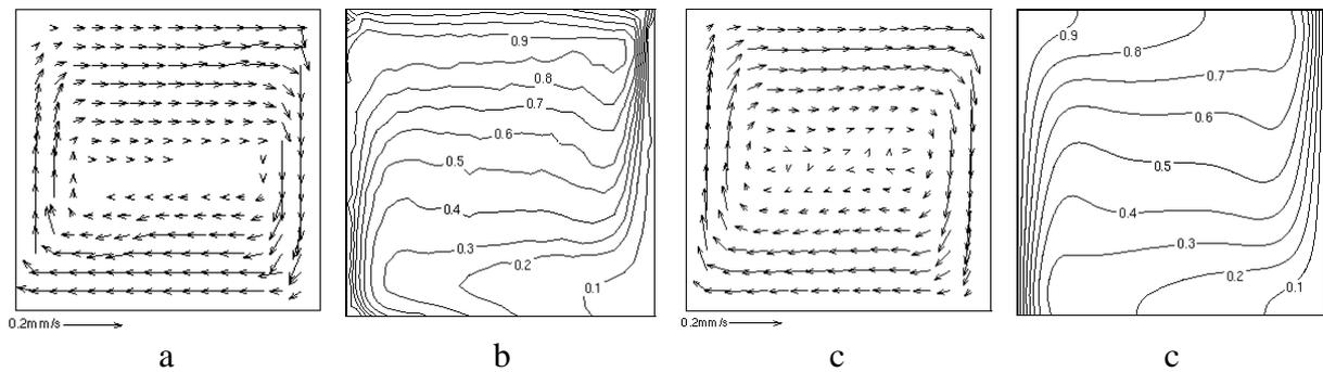
**Figure 7.** DPIV (a) and DPIT (b) measured velocity and temperature fields for natural convection in centre plane of differentially heated cavity; numerical counterparts (c) and (d).  $Ra=1.7 \cdot 10^5$ ,  $Pr=1109$
