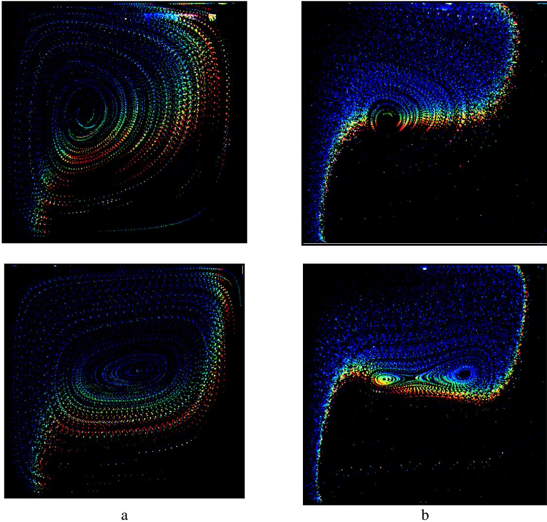
**Figure 6.** Multiexposed photographs of liquid crystal tracers in the convective flow at the front wall  $z=0.95$  (top row) and the centre plane  $z=0.5$  (bottom);  $Pr=6300$ . Effect of Rayleigh number: (a)  $Ra=2 \cdot 10^4$ , (b)  $Ra=8 \cdot 10^4$
