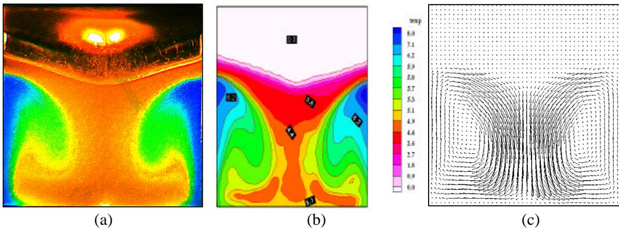
**Figure 12** Freezing of water from the top in the lid cooled cavity. Recorded image of TLC tracers (a), evaluated temperature (b) and velocity (c) fields. Time step - 3600s after cooling starts;  $T_c = -10^\circ\text{C}$ ,  $T_{ext} = 20^\circ\text{C}$ ,  $Ra = 3 \cdot 10^6$ ,  $Pr = 13.3$
