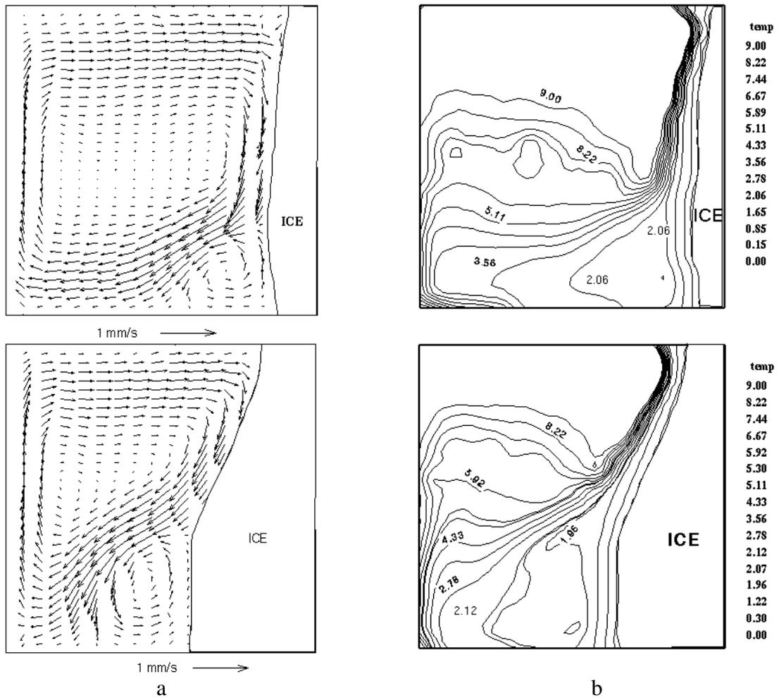
**Figure 10.** DPIV (a) and DPIT (b) measured velocity and temperature fields for natural convection in centre plane of differentially heated cavity at 500s (top) and 3000s (bottom).  $T_h=10^\circ\text{C}$ ,  $T_c=-10^\circ\text{C}$ ;  $Ra=1.5 \cdot 10^6$ ,  $Pr=13.3$
