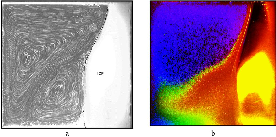
**Figure 9.** Visualization of natural convection in freezing water. Particle tracks showing flow structure (a), liquid crystals tracers indicating variation of temperature (b).  $T_h=10^\circ\text{C}$ ,  $T_c=-10^\circ\text{C}$
