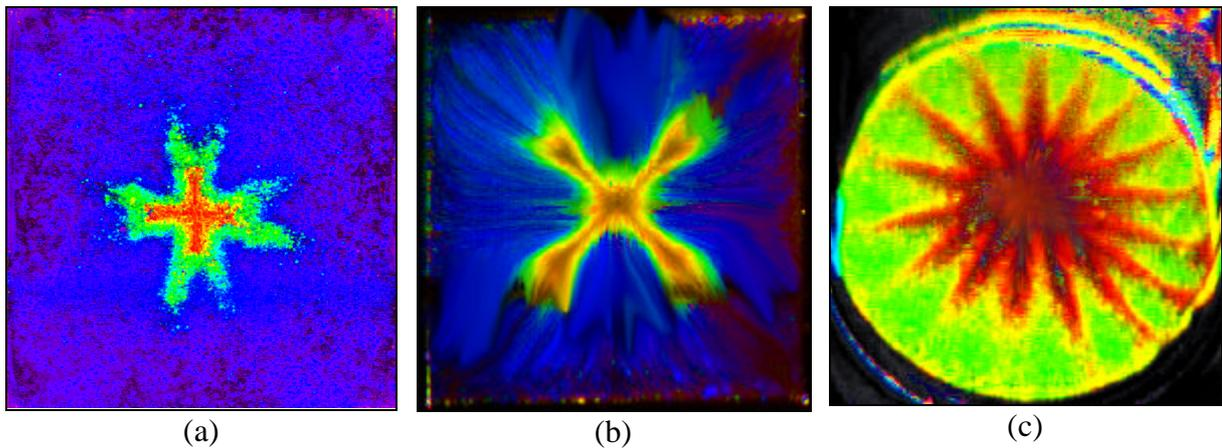
**Figure 13.** Natural convection in the lid cooled cavities. Temperature distribution recorded with help of TLC directly under the cooled top wall. Effect of the walls properties on the flow structure visible in the temperature fields: (a) - plexiglas walls, (b) - glass walls, (c) - cylindrical glass cavity
