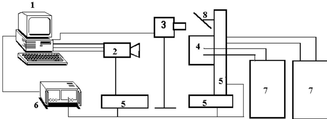
**Figure 3.** Schematic of the experimental system. PC (1) with the acquisition card controlling RGB camera (2), halogen lamp (3) and three stepping motors (5) using driver (6). Temperature in the cavity (4) controlled by two thermostats (7); mirror (8) used to direct light sheet
