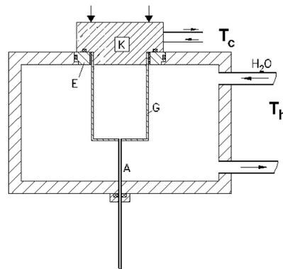
**Figure 5.** Lid cooled cavity, schematic of heating for the lid cooled cavity with an isothermal top lid (K) immersed in the external hot water bath
