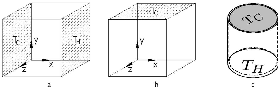
**Figure 4** Investigated geometry: differentially heated (a), lid cooled cube (b) and cylindrical cavity (c)
