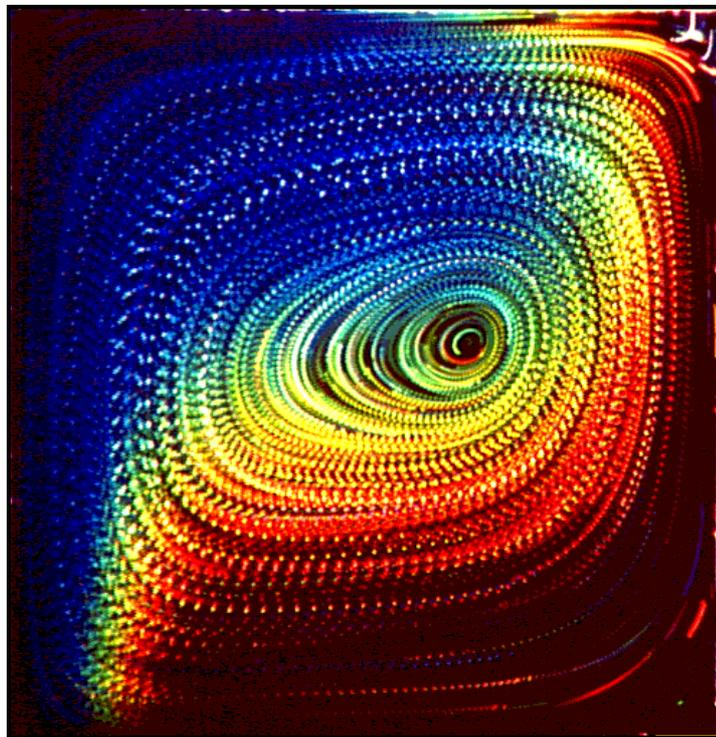
**Figure 1.** Multiexposed colour photograph of the convective flow in glycerol seeded with liquid crystal tracers in a differentially heated cavity. Tracers change colour from blue to red following the clock-wise flow circulation from the hot wall (left) to the cold wall (right); temperature difference  $\Delta T=4^{\circ}\text{C}$ ,  $Ra=1.1 \cdot 10^4$ ,  $Pr=6900$
