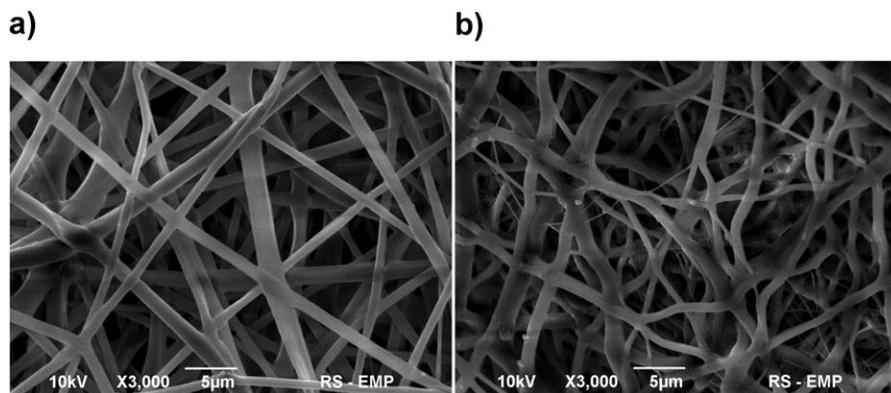
**FIGURE 4.** Comparison of SEM micrographs of two materials made from two polymers by emulsion electrospinning: a) PDLG polymer—M3, b) PLC polymer—M4.
