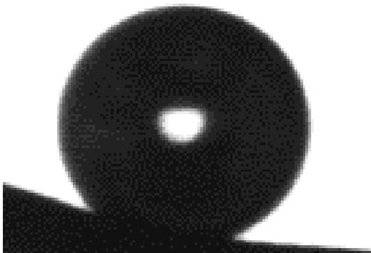
Fig.5. Cropped image of the alcohol vapour bubble growing at the wire. Bubble diameter is 0.2mm.
