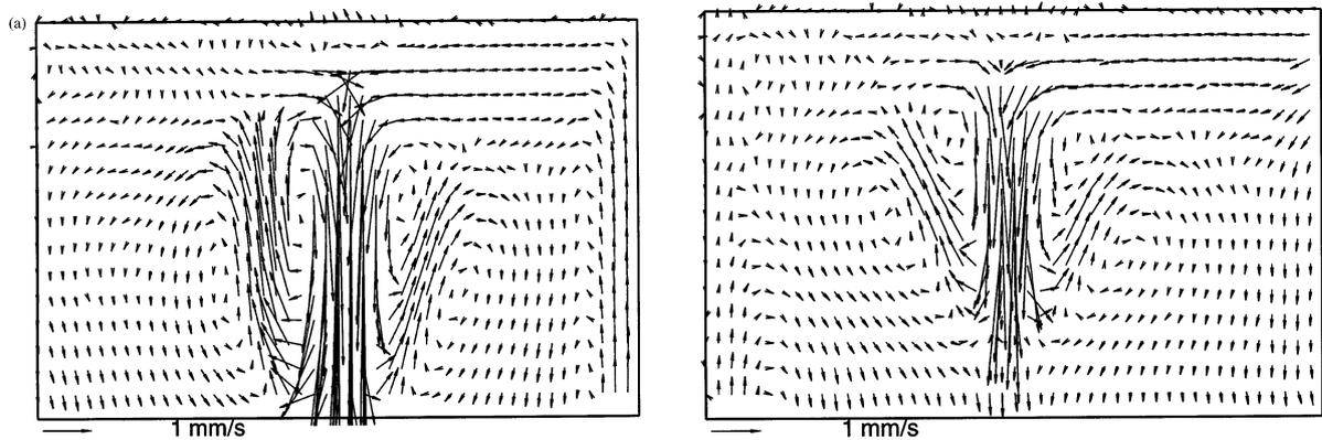
Fig. 7. Measured velocity field in the centre cross-section by DP-PIV method; only every 16th vector displayed. (a) Plane beam, horizontal size 62 mm, (b) focused beam, horizontal size 53 mm.
