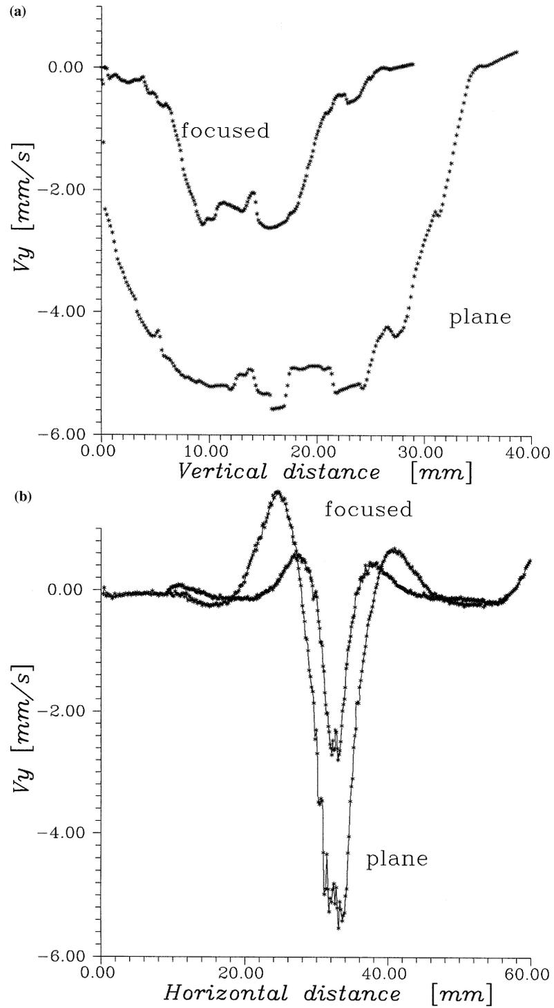
Fig. 8. Velocity profiles extracted from the PIV measurements. (a) Vertical velocity component along transducer axis, distance measured from the transducer external surface, (b) vertical velocity component along horizontal line, passing maximum value (approximately 17 mm from the plane transducer and 13 mm from the focused one).
