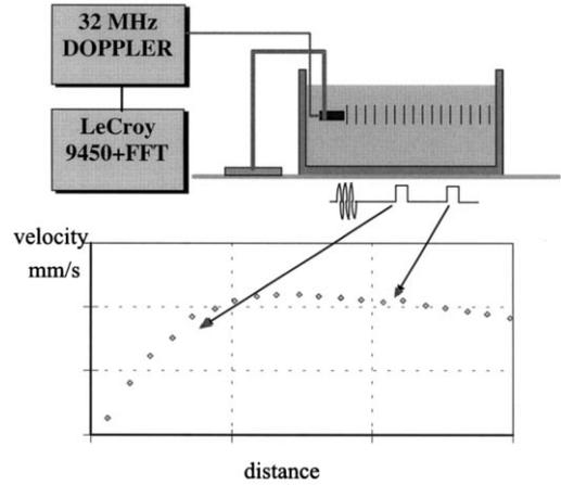
Fig. 1. Block diagram of the Doppler measurement set-up.
