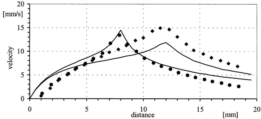
Fig. 5. Streaming vs. distance; focused transducers, focal distance = 8 and 12 mm, radius of the transducer is equal to 4 mm. The solid line, theoretical calculations, points, experimental results (Nowicki et al., 1997).
