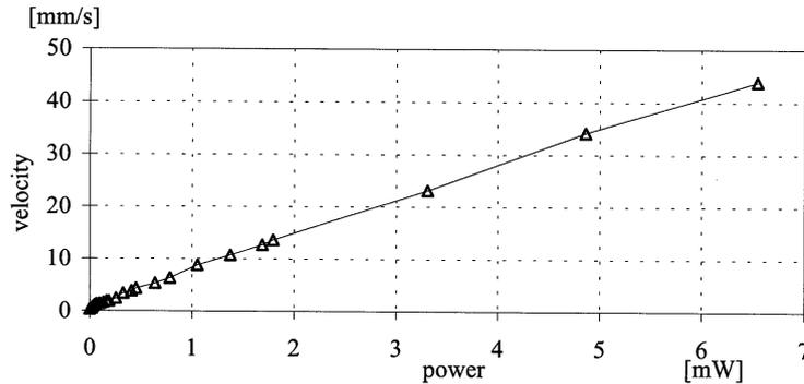
Fig. 2. Streaming velocity in function of the radiated acoustic power; plane 32 MHz transducer (Nowicki et al., 1997).
