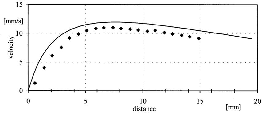
Fig. 4. Streaming velocity vs. distance, plane 32 MHz transducer. The radius of the transducer is equal to 4 mm. The solid line, theoretical calculations, points, experimental results (Nowicki et al., 1997).
