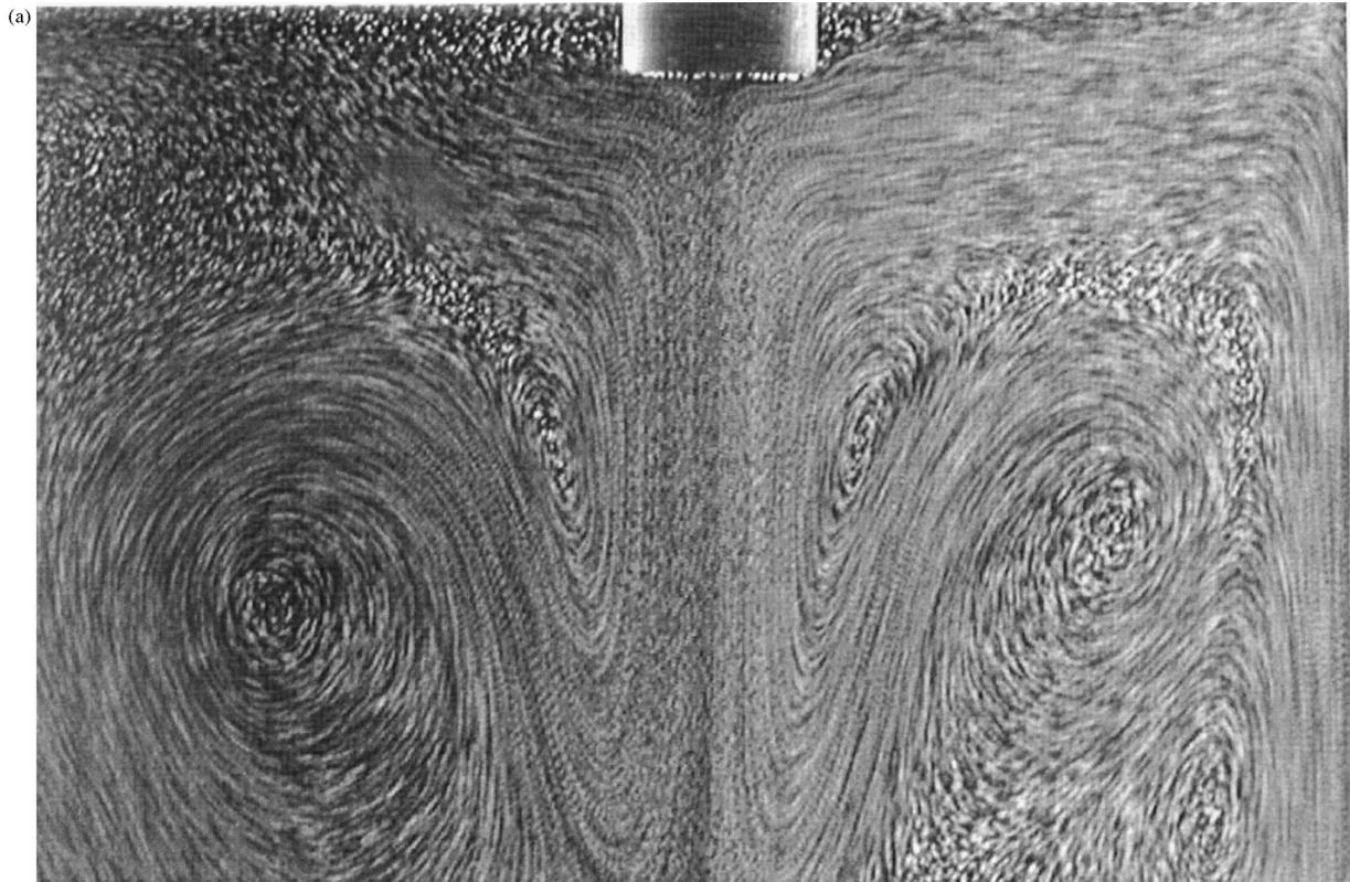
Fig. 6. Visualisation of acoustic streaming, ten superimposed images taken at 200 ms interval. (a) Plane wave transducer, (b) focused transducer.
