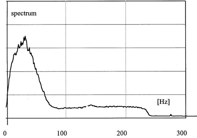
Fig. 3. Doppler spectrum of the streaming velocity measured at the depth of 0.6 mm for plane beam.
